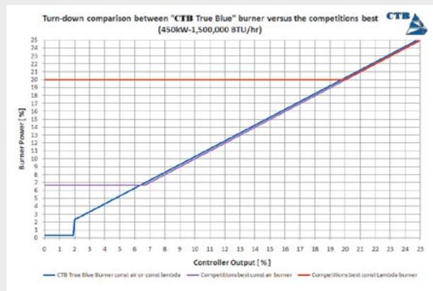
line) is necessary for good temperature uniformity as well as for the firing atmosphere. Burners that do not cover the lower control range are not suitable for this model process.
