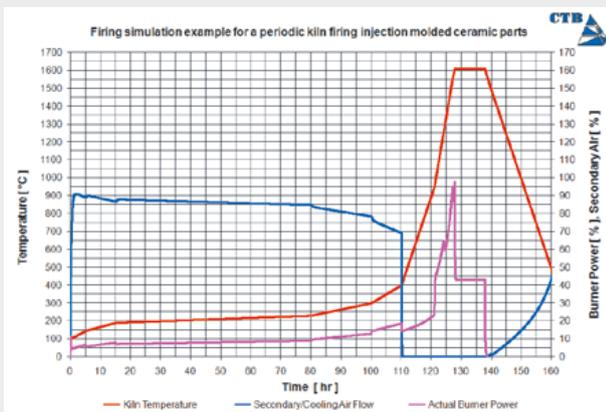
Chart 1: For a defined optimum firing curve (red line), the energy requirement of the burners in the first 80 hours of the firing cycle is well below 10 % of the burner capacity. The volume of secondary/diffusion air shown here (blue
